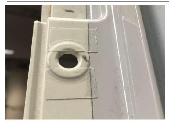
5. Reinstall the 2 T-nut screws per side, torque to 14 Nm.
