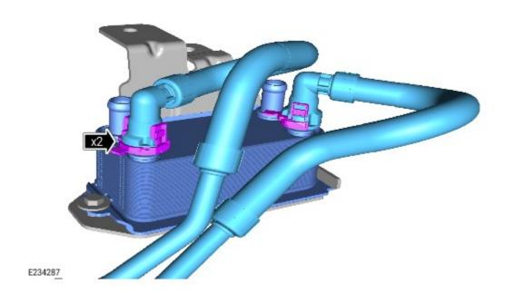
Install the new transmission fluid cooler pipes to the transmission fluid cooler.
