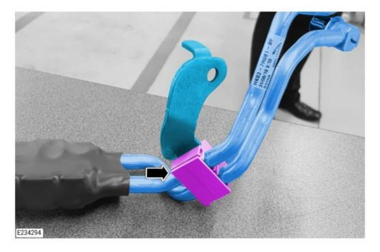
Remove the bracket from the **NEW** Transmission fluid cooler pipes (T4A29688).
