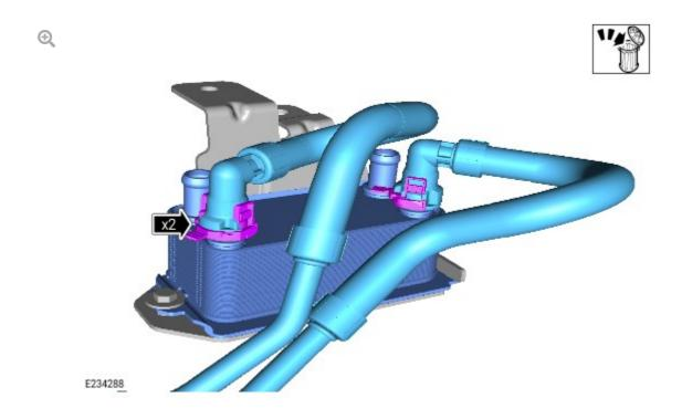
Remove and discard the transmission fluid cooler pipes.
