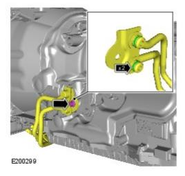
Install the transmission fluid cooler pipes.
