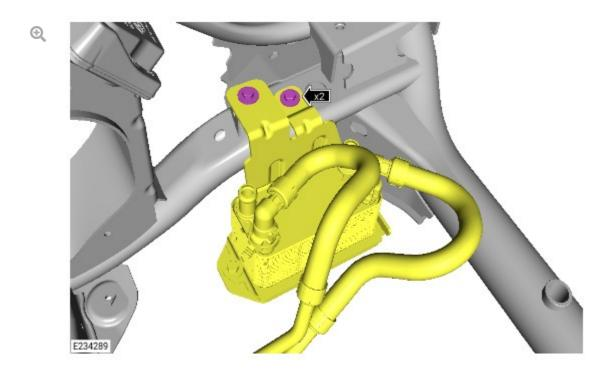
Release the transmission fluid cooler assembly from the front subframe.
