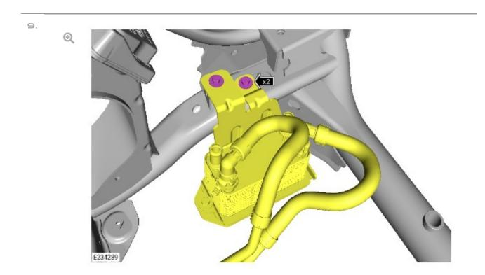
Install the transmission fluid cooler assembly to the front subframe.
