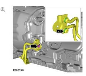
Release the transmission fluid cooler pipes.
