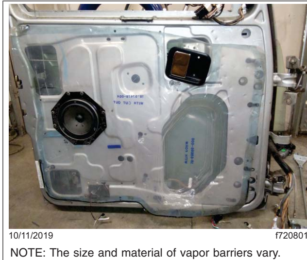
Fig. 4, Example of Vapor Barrier
