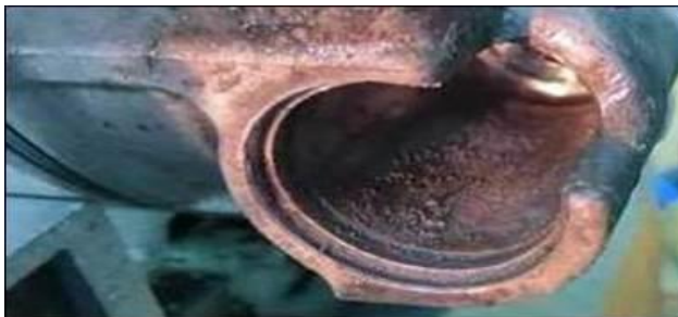
Figure 11. Corrosion in the N280 valve bore.
