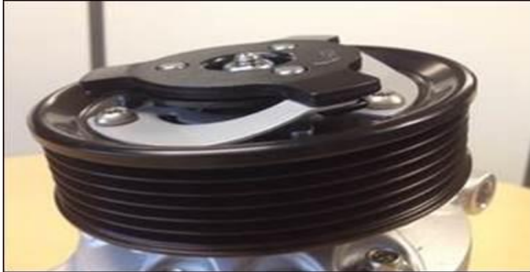
Figure 5b. Example of torque limiter over load protection still intact.
