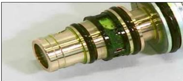
Figure 12: Severe contamination at the N280 valve filter screen.
