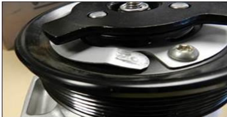
Figure 5a. Example of torque limiter over load protection
