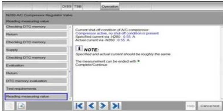
Figure 3. Checking N280 signal value Measuring Value Block.
