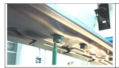
C. Use cartridge gun 83 19 2 149 522 to apply K5a body adhesive around the **side** of each bushing as shown.
