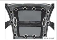
Remove the rear sunroof glass panel following repair instructions REP 54 13 250 "Removing and installing/replacing rear glass slide/tilt sunroof panel". The front glass slide/tilt sunroof will be removed at the same time.
