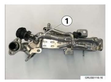
9. Check the bypass flap on the EGR cooler.
