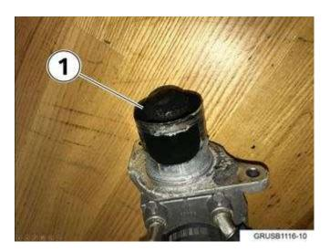
Remove the EGR valve and check for jamming (1) (valve is normally sprung closed).
