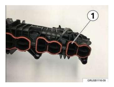
Check all swirl flaps for damage or melting/missing parts (1).
