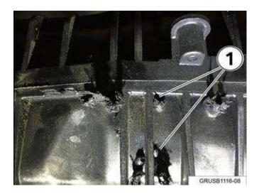
Are there visible signs, on the intake manifold and venturi pipe, of overheating, similar to the illustration (1)?
