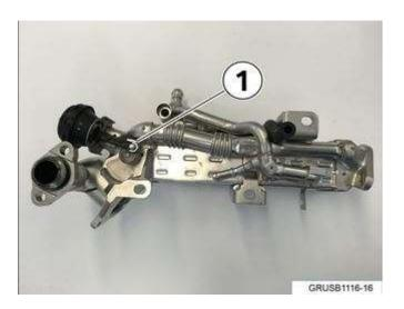
Check the bypass flap on the EGR cooler.
