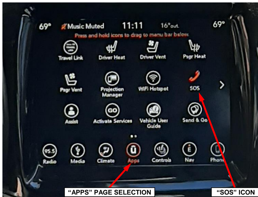
Figure 1 – Connected Services Enabled
