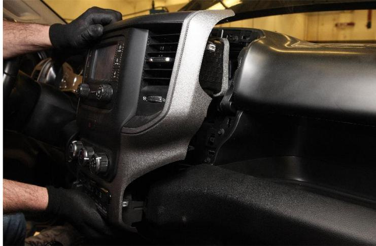
**Figure 5 – Instrument Panel Center Bezel**
