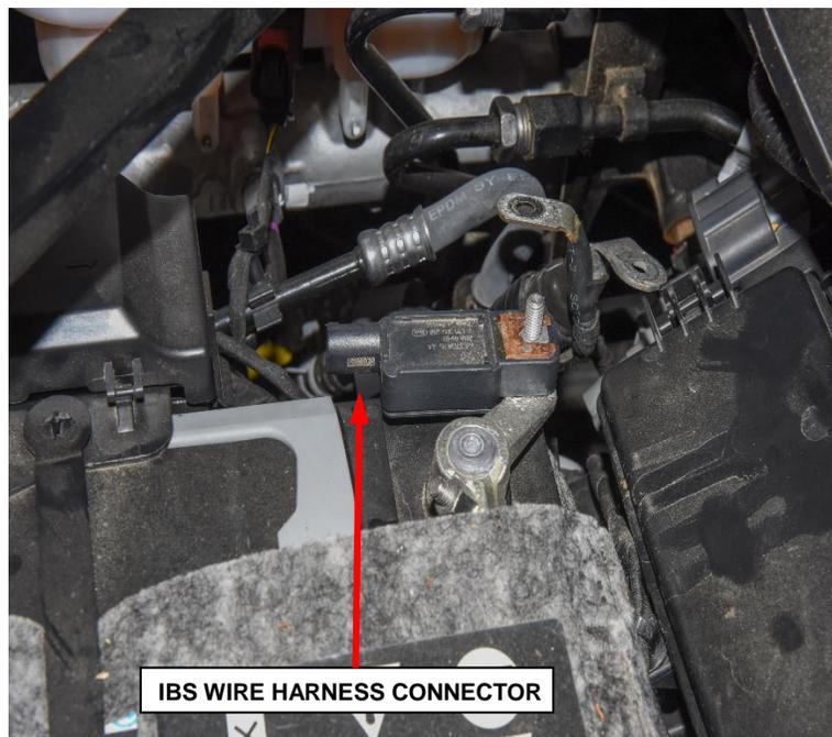
Figure 1 – IBS Wire Harness Connector
