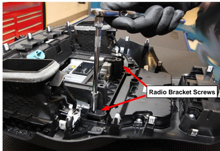
**Figure 9 – Radio Bracket Screws**
