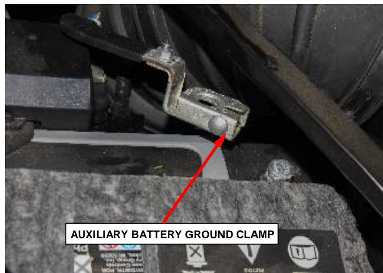
**Figure 3 – Auxiliary Battery Ground Clamp**
