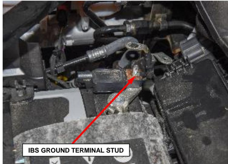
**Figure 2 – IBS Ground Terminal Stud**
