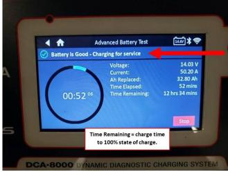
In the post-test charging mode, the DCA analyzes the current state of charge of the battery and automatically begins to charge the battery to a fully charged condition, 100% state of charge. The time required to charge the battery to full will vary.
