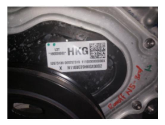
As shown in the abovephotos, the engine broadcast code can be found on the engine front cover just above the harmonic balancer
