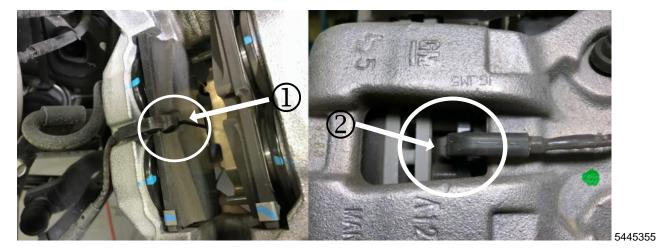
5. Inspect the brake pad wear sensors on both the front (1) and rear (2) brake pads. Remove the front brake caliper to gain a clear view of the brake pad wear indicator for inspection as shown.
