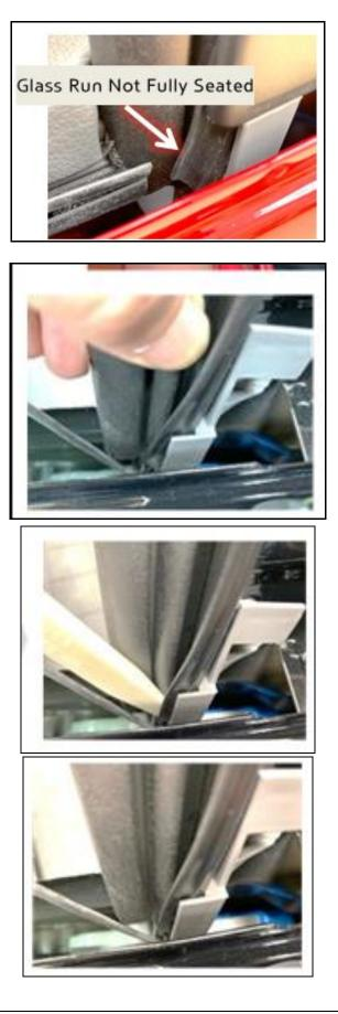
2. Use a nylon/plastic trim removal tool to fully seat the glass run.
