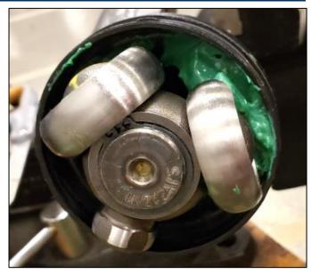
22. Install a provided new circlip into the CV cup.
