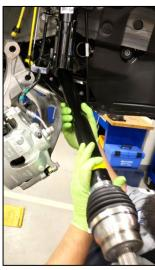
12. Remove the circlip on the end of the axle shaft, transmission side.
