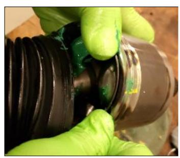
23. Seat the CV boot onto the cup.
