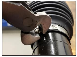
Remove the large band clamp using the OTC CV band clamp tool and a small flathead screwdriver.
