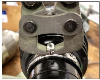
26. Install a provided new circlip onto the end of the CV shaft.
