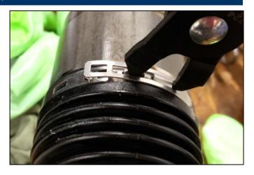
25. Secure the small CV band clamp using CV Band Clamp Tool SST 09495-3K000A by pinching the ear together.
