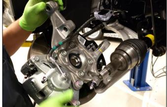
9. Support the knuckle assembly using a bungee cord, hanger, or similar to minimize strain on the brake caliper line.
