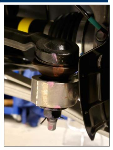
6. Use Ball Joint Remover SST 09568-2J100 to separate the tie rod end ball joint and release the tie rod end from the knuckle.
