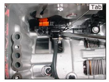
14. Remove two bolts that secure the harness to the case.
