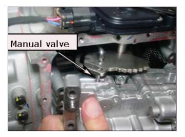
17. Install the valve body bolts and torque the bolts to specification from the center bolts to the outermost bolts.
