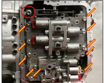
18. Connect the new oil pressure harness to the solenoids and install the oil pressure sensor.
