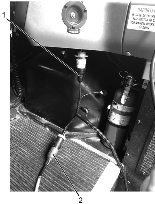
Figure 5. Powerlink Programming Cable - USB Interface
