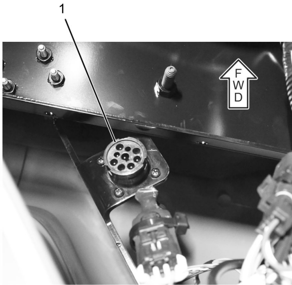
Figure 3. Data Link Connector (DLC) - Under Dash
