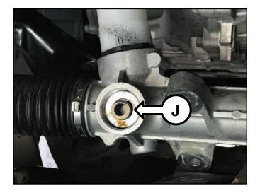
17. Partially install the new yoke plug (L) by <u>hand</u> to prevent cross-threading of the plug and housing threads.
