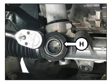
Using the 24mm hexagon bit socket (HXD24), remove and discard the yoke plug (I) and discard.
