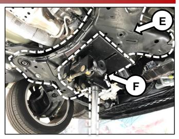
5. Remove the two (2) subframe retaining nuts (G) and carefully lower the subframe.
