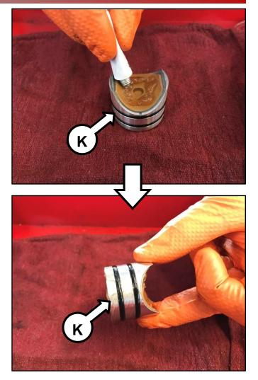
Install the improved yoke assembly (K) into the yoke housing and then apply a small amount of lubricant to the top of the yoke assembly.
