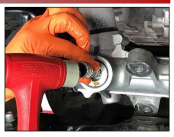
16. Reinstall the yoke spring (J) removed in step 10 of this procedure.
