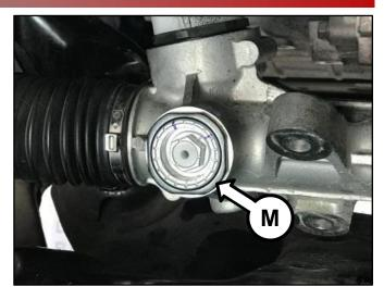
22. While holding the plug in place, torque the locking nut (M) to specifications.
