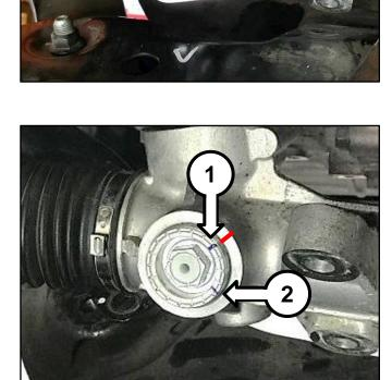
20. Loosen the plug approximately 1/4 of an inch and align the mark on the housing with groove 2 (blue mark #2) of the plug.
