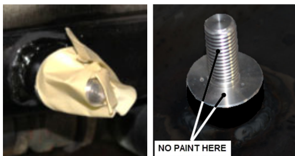
FIGURE 78: GROUND STUD #380360
