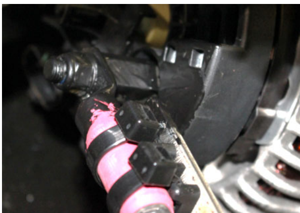
FIGURE 134: POSITIVE (+) CONNECTION ON THE ALTERNATOR
