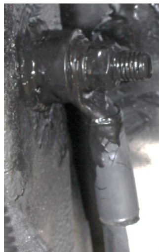
FIGURE 122: GROUND STUD WITH RUBBER COATING
