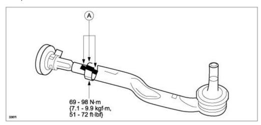
9. Install the steering gear and linkage (both sides) according to the instructions on MGSS online:
