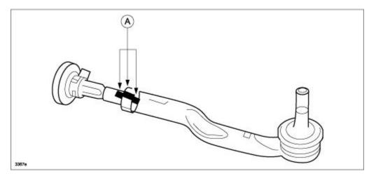
b) Insert a flathead screwdriver into the boot band (as shown below), then press the caulked area outward to remove the boot band (both sides).
