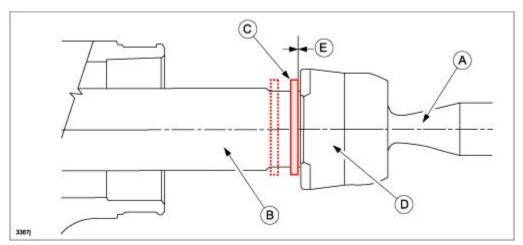
7. Reinstall the boot using a new boot band from the joint set (both sides) according to the instructions on MGSS online:
