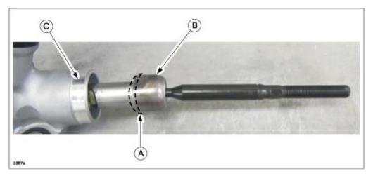
To eliminate the noise, a spacer (A) has been installed between the inner ball joint (B) and the steering gear housing (C) (both sides) to prevent direct contact.
