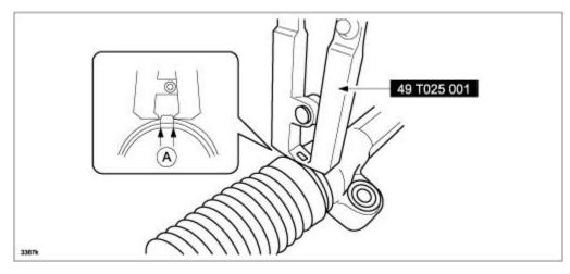
8. Align the alignment marks (A) made before removal and assemble the tie-rod end to the tie rod (both sides).
