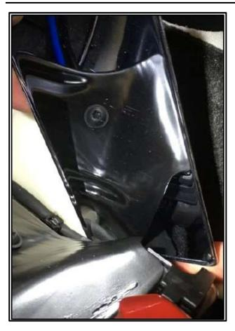
Check outer backrest frame with an inspection mirror.
