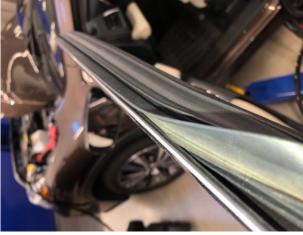
• Plastic "T" clips are used to secure the weatherstrip to the lower portions of the door. **CAREFULLY** pull (stretch) the weatherstrip one way only as far as needed to release it from one side of the "T" clip then slide it off the other side. **NOTE:** The replacement weatherstrips have new "T" clips already installed.
