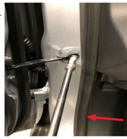
• Pull the weatherstrip out of the retaining grooves securing it to the upper half of the door.
