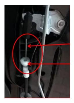
2. Visually inspect the Bowden release cable for the inner door handle of the affected door(s) for signs or water or corrosion in the area circled.
