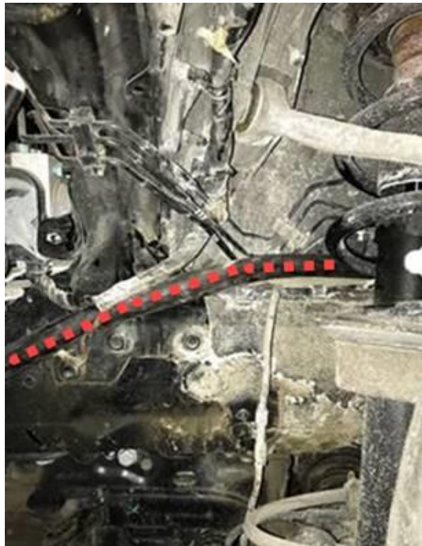
Figure 5. Route the 5/8" ID rubber hose from new filter position to the J909.
