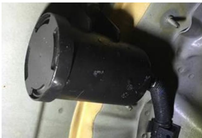
Figure 2. Ventilation tube of the EVAP canister.
