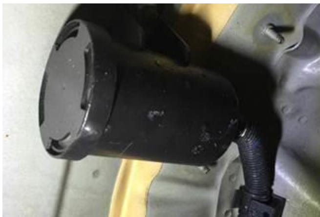
Figure 10. Remove original NVLD filter.
