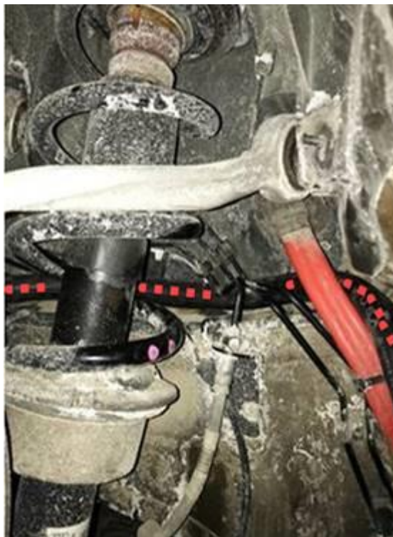
Figure 6. Routing the rubber hose.
