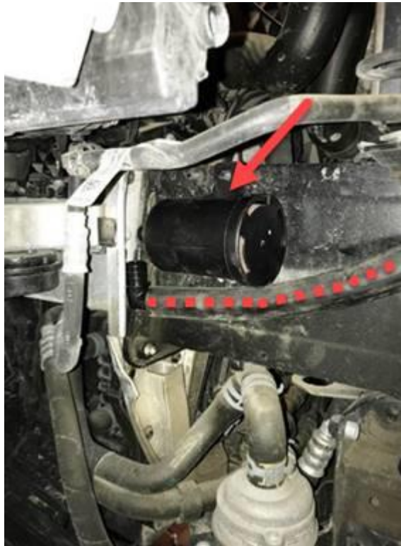
Figure 3. Installing the new NVLD filter.
