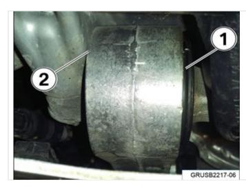
The bushing in the lower engine stabilizer link (1) is working its way out of its aluminum housing. The aluminum housing starts to rub against the engine oil pan (2).
