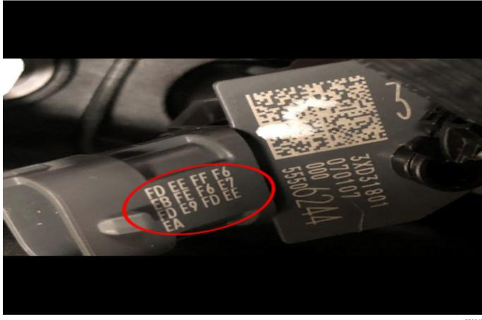
If the injector flow rate identifier labels have been removed from the OEM and/or Service engine, use the injector flow rate identifier written on each injector
