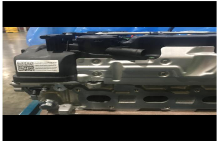
The Service Engine has an injector flow rate identifier label located on the side of the camshaft cover. This label is only valid as long as all original 6 injectors are still installed in the engine. If a fuel injector requires replacement the label must be removed and discarded 5568473
