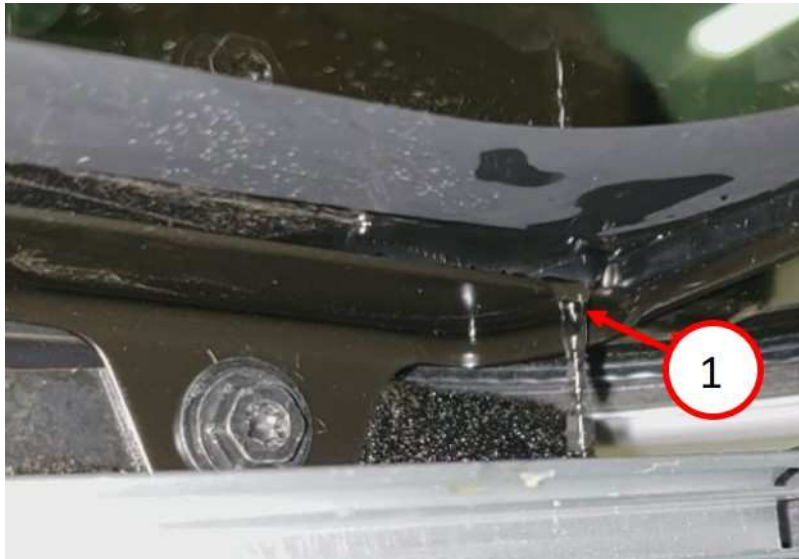
Fig. 5 Example of Water Leak
