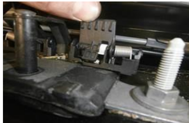
Figure 3. Debris in the rear lid closed sensor.
