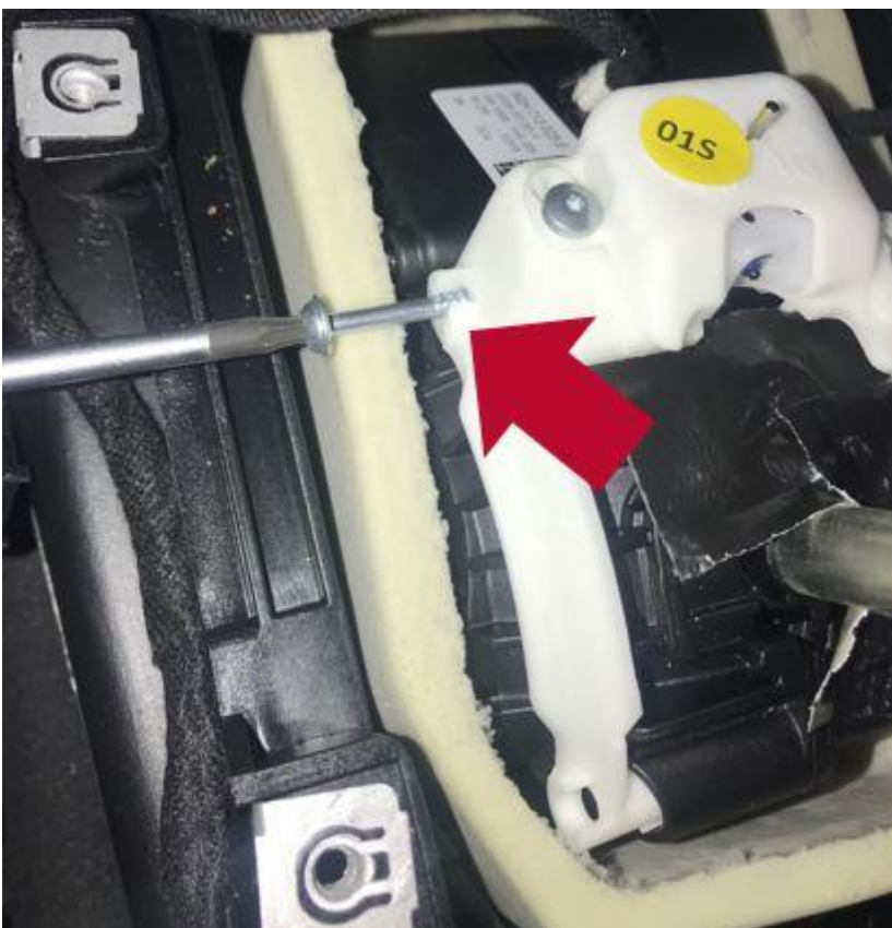
Figure 8. Installation of the screw.
