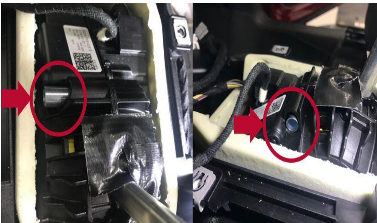
Figure 5. Installing the spacer sleeve.
