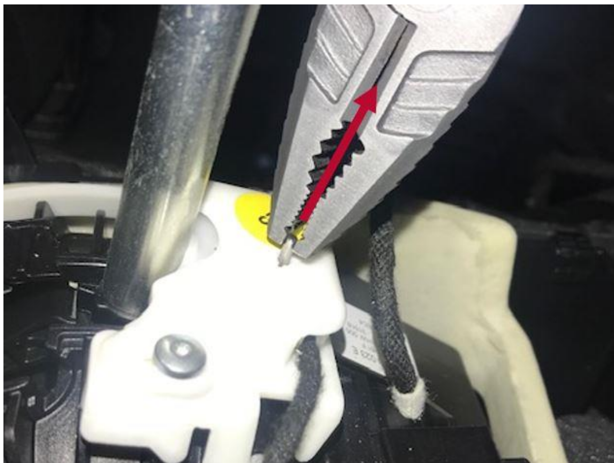
Figure 11. Removing lock pin from the microswitch module.
