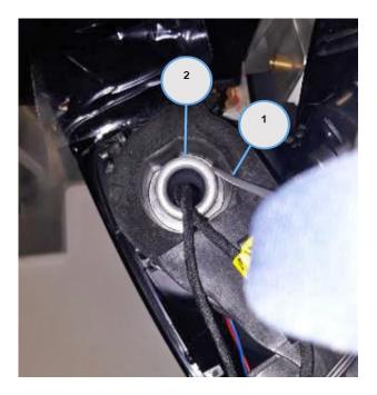
2. Using special lubricant, P/N 83 19 9 408 523 (1), apply lubricant to all visible surfaces of the sliding disc (2) as shown.
