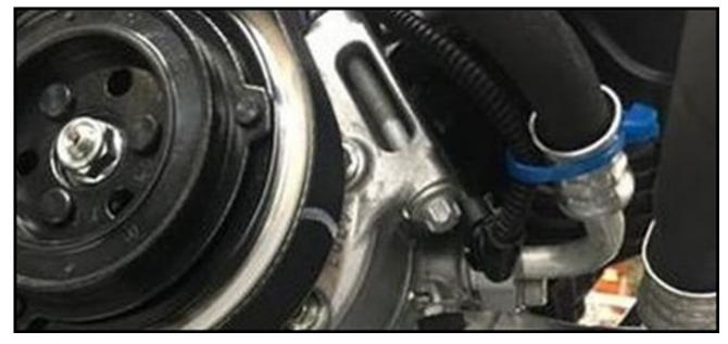
**Note:** Only the heat-resistant cable tie must be used to secure the wiring harness to the metal crimp of the air conditioning refrigerant line as shown above.
