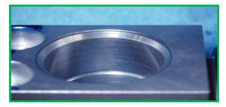
Damage – **No Good Part**Expansion valve seal bore is damaged due to deep scratching perpendicular to O-ring groove.
