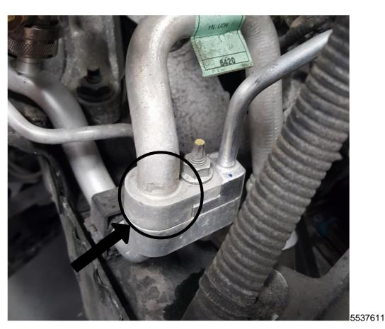
• Be sure to replace the accompanying A/C Compressor Hose Seal (circled above) while replacing the Condenser Hose.
