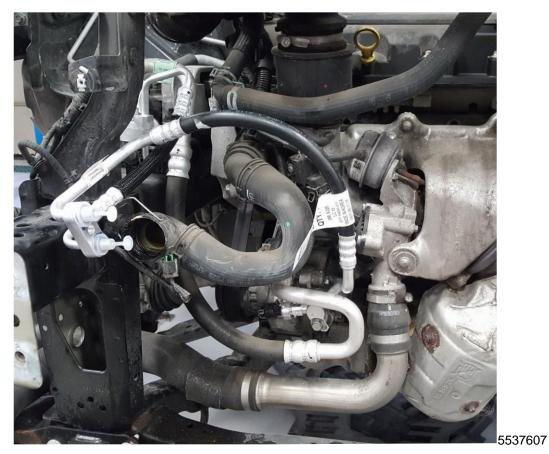
15. Replace the Air Conditioning Condenser Hose with the new part provided as shown.
