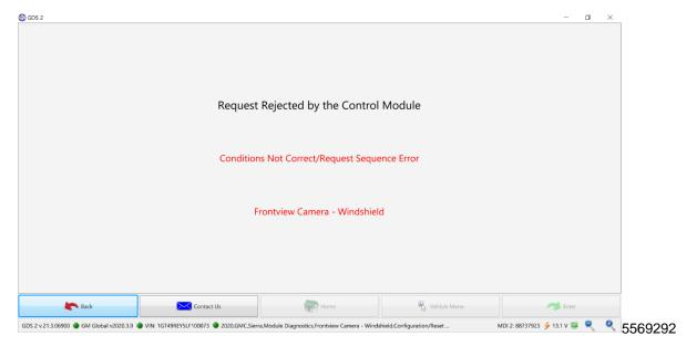
1.5. In the event if you receive this screen after Selecting Reset Button then the Camera was not in learn mode. To ensure this, confirm if DTC B0395D is in History. If so, Exit GDS2 and continue to step 2.
