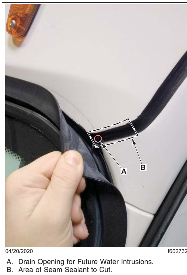
Fig. 3, Seam Sealant Opening and Area to Cut
