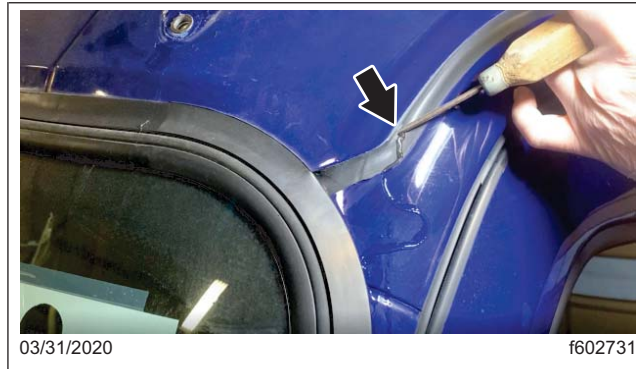
Fig. 2, Draining Collected Water
