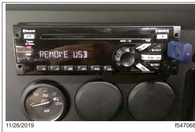
Fig. 5, Radio Displaying "Remove USB"
