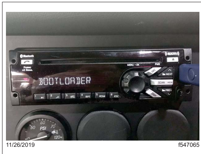
Fig. 3, Radio Displaying "Bootloader"
