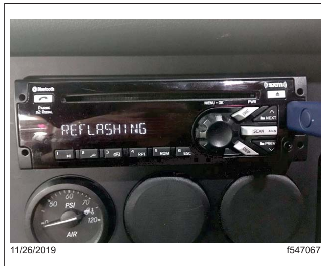
Fig. 4, Radio Displaying "Flashing"
