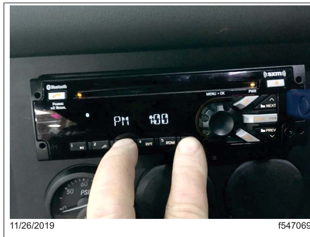
Fig. 2, Holding Buttons 3 and 6
