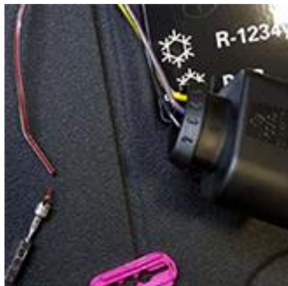
Figure 1. T4e with damaged wire.
