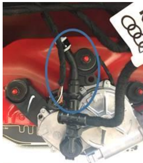
Figure 3. Check valve assembly installed.
