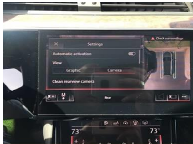
Figure 1. Clean rearview camera function being displayed.
