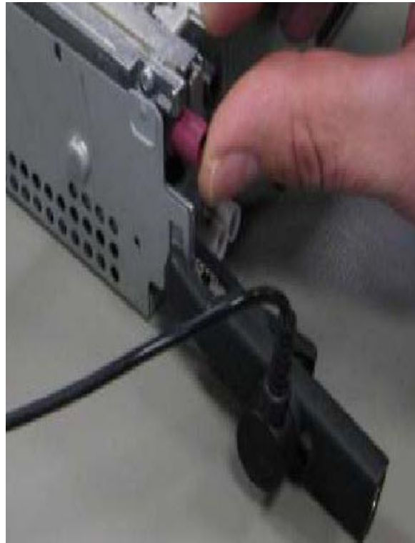
Figure 7. Alligator clip on the MMI housing.
