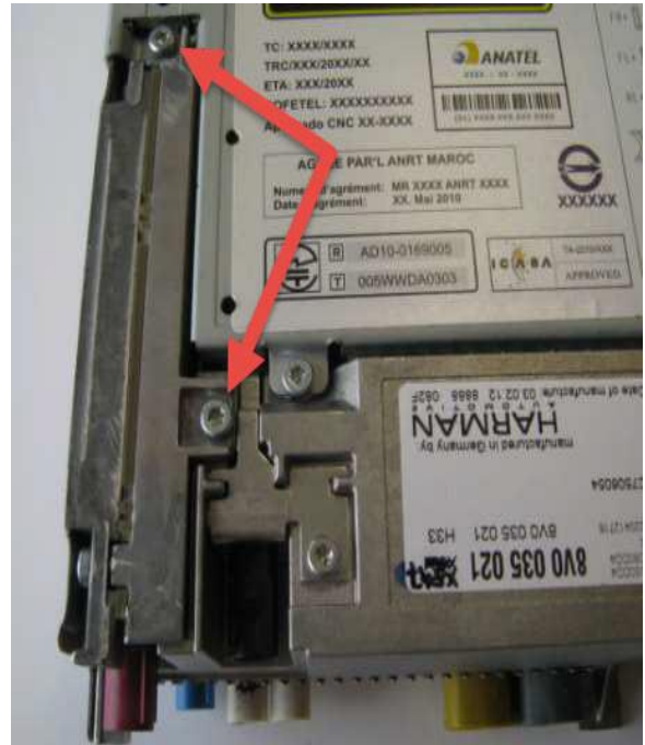
Figure 13. Do not over-torque screws.
