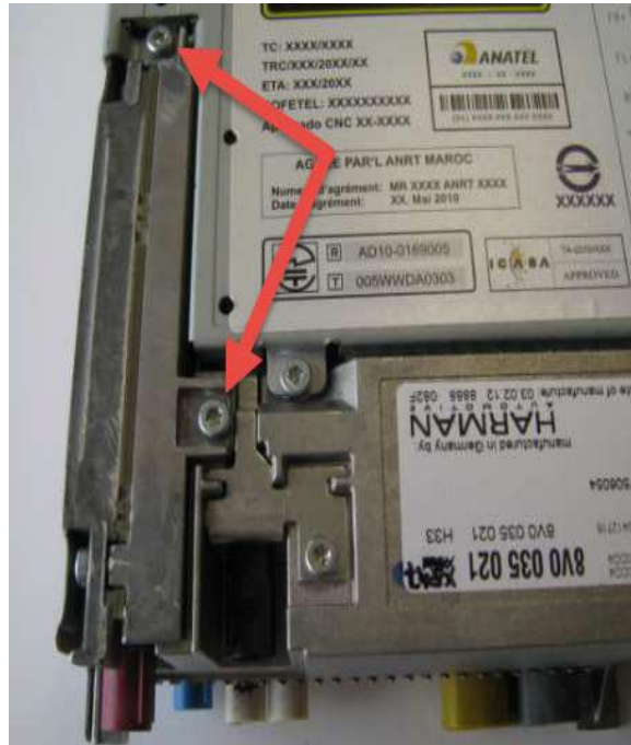
Figure 9. Telephone module screws.
