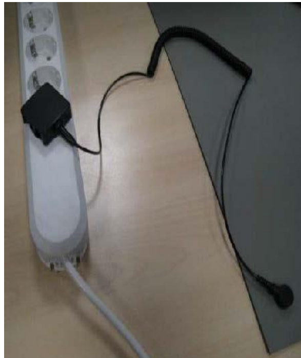
Figure 4. Grounded ESD work surface.
