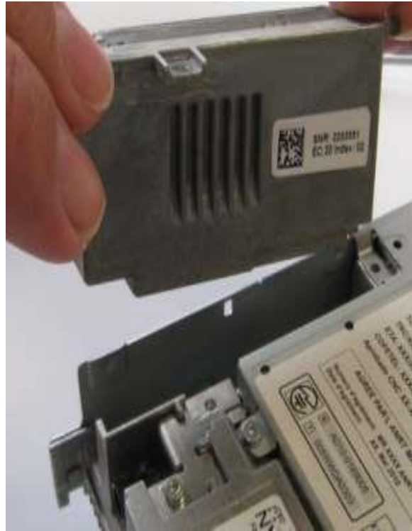
Figure 12. Insert the new telephone module.
