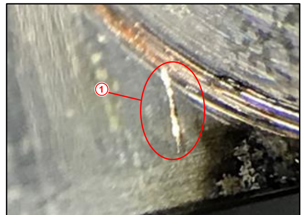
1 Debris Created From Bolt Tightening
