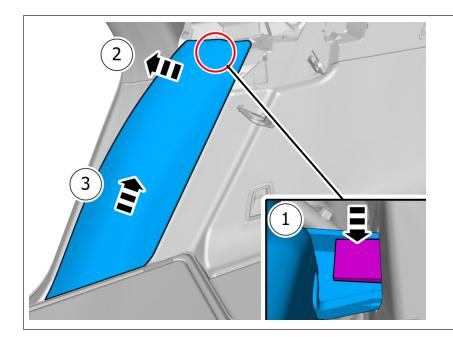
Release the catch. Remove the marked part.
