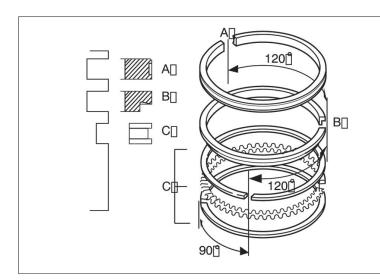
Caution! Make sure that the piston rings can be easily rotated by hand in the piston ring grooves.
