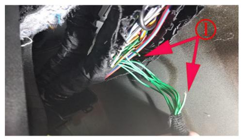
If an open is found repair the circuit following SI Serial Data Circuit Wiring Repairs.
