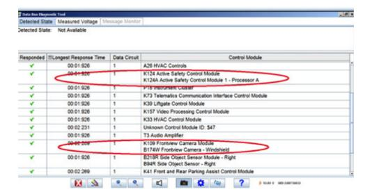
If it is found that the K124 ASCM is not communicating on low speed (with UGN) inspect circuit 5060 for an open in the harness near JX300.
