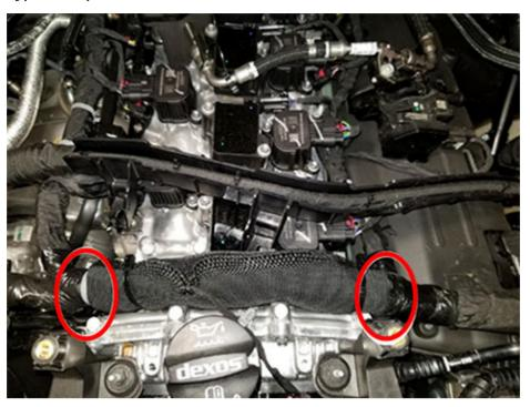
**Example of engine wiring harness damage at Camshaft Carrier Cover shown below.**
