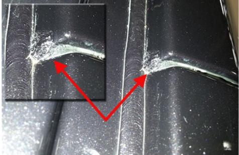
6 - With the roof rail removed on the affected side, inspect existing seam sealer in the area shown; door surround to quarter panel and roof panel (Area 2 as seen above) for skips or pin holes in the sealer.
