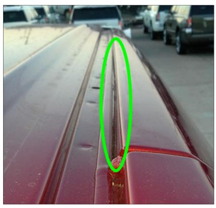
8 - With the roof rail removed on the affected side, inspect existing seam sealer in the area shown; quarter panel to roof panel (Area 3 as seen above) for skips or pull-away along the outboard edge.
