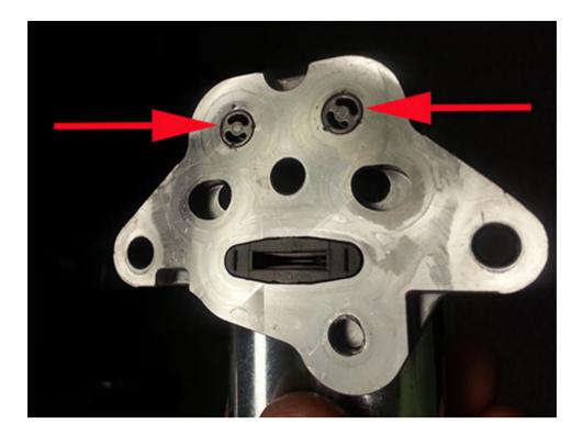
This is a bad valve with components missing.
