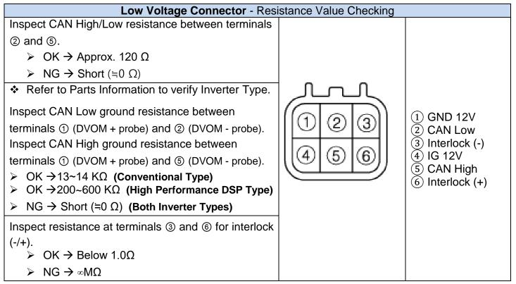
**NOTE:** Connect the high voltage connector in order to measure the interlock resistance.
