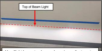
Headlight beam too low and requires adjustment upward to the line on the wall which is 26.2 inches high.
