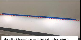
Headlight beam is now adjusted to the correct height and specification.
