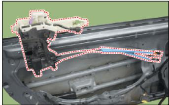
2. Locate the drain hole located at the bottom of the door latch assembly.
