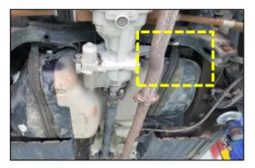
2. Using a rubber/plastic hammer, place the bottom end of the hammer against the canister surface and while holding firmly, tap the head of the hammer five (5) times and listen for loose charcoal sound from inside the canister.
