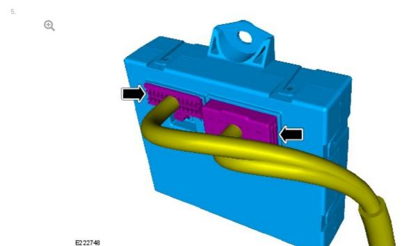
Disconnect the power tailgate module and position the electrical wiring harness to one side.
