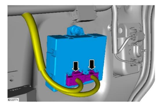
Connect the electrical wiring harness to the power tailgate module.
