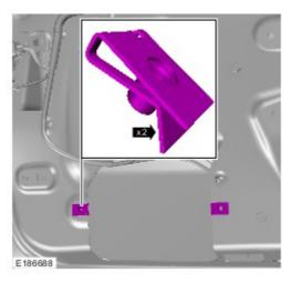
Install 2 new retaining clips (AYH100790).
