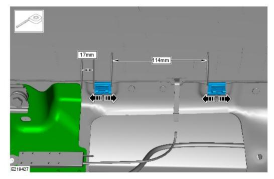
Adjust the position of the new tailgate clips as shown.
