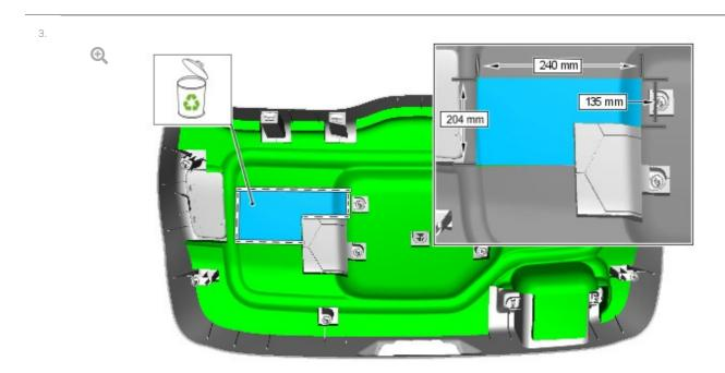
Use a suitable knife to carefully remove a section of the Noise, Vibration and Harshness (NVH) material from the tailgate trim panel, as shown in the illustration.
