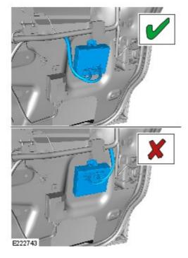
The power tailgate module must be installed with the electrical connectors towards the bottom of the tailgate.
