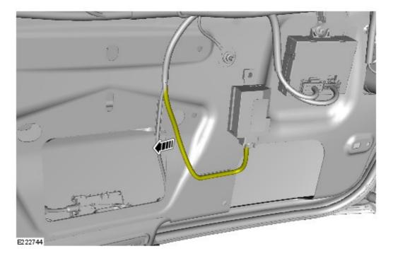
Position the wiper relay suppression module wiring harness to the side.
