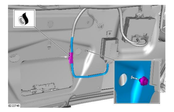
Secure the wiper relay suppression module wiring harness to the tailgate wiring harness with suitable electrical tape.
