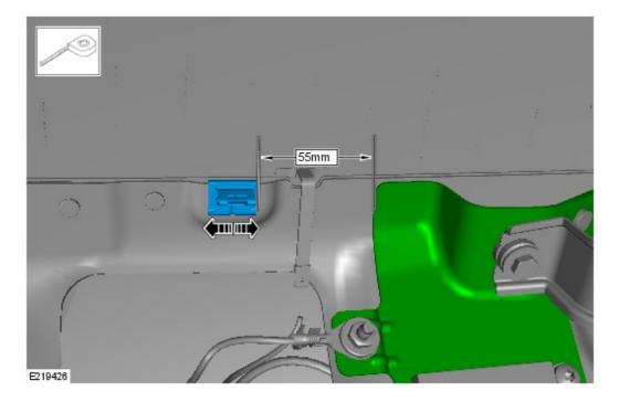
Adjust the position of the new tailgate clip as shown.
