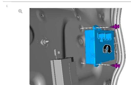
Remove the power tailgate module and rotate through 180 degrees.
